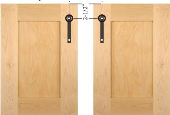
Place top hardware hole 2-1/2" from top of rail and center hardware horizontally on stile. On individual doors place hardware on right side stile as shown above left. On pair of doors place hardware on adjacent stiles as shown above.
