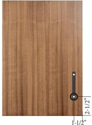
Place knob or pull 1-1/2" from right or left edge of door and 2-1/2" up from bottom of door.
