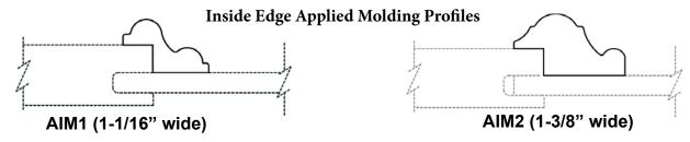
Inside edge applied moldings are available on cope and stick door styles using FP3/8", RPAM1 or RPAM2 and any outside edge.
