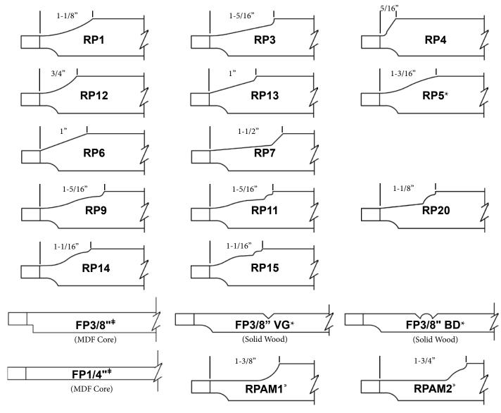
\*RPAM1 and RPAM2 are for use on Inside Applied Molding Doors. Reveal varies depending on which applied molding is used.
